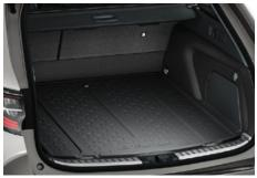
**BOOT LINER**Tailored to fit the boot of your vehicle and provide protection against dirt and spills.
