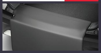
The rear bumper protection apron is fixed to the trunk deck with velcro. It protects the rear bumper when unfolded.
