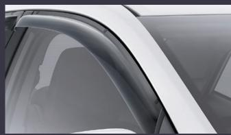
\*Front and rear available for €195.00 Wind deflectors are ideal if you like to drive with the windows open. They are custom designed to match the aerodynamic contours of your vehicle and work by diverting airflow to ensure that you and your passengers are not troubled by excessive wind movement and noise.
