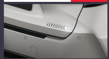
Rear parking sensor system with 4 ultrasonic sensors and an acoustic warning.
