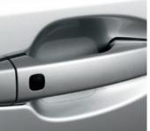
DOOR HANDLE PROTECTION FILM The door handle protection film is tough transparent self-adhesive film that helps protect door paintwork against those small scrapes and scratches.
